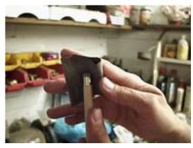
PHOTO: Be careful to angle the sandpaper away from the cue so that on your downward strokes you don't scratch the ferrule and, more importantly, you don't scratch the shaft of the cue.
