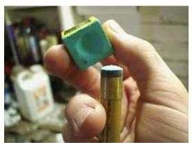
PHOTO: This is the sort of shape your new tip should have. Not too rounded and not too flat, just a nice gentle dome.
