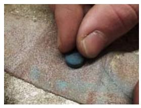
PHOTO: Try to keep the tip flat as you sand it. If you 'rock' it you will make the surface convex or angles and cause problems when glueing.
