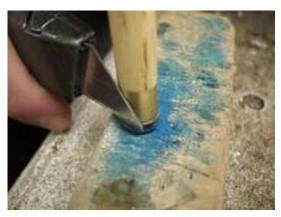
PHOTO: Carefully cut away the overhanging tip making sure you keep the blade as vertical as possible thereby 'sliding' down the ferrule, using it as a guide, and cutting the tip flush and level. Don't cut or scratch the ferrule.
