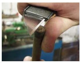
PHOTO: REMEMBER - You are not trying to make the surface flat with the blade because it should already be flat. You are just trying to remove anything still stuck to the surface. NOTE: If you do not ensure that the surface is perfectly flat, you will probably have problems getting the tip to stick. If it does stick, the chances are that it will fly off shortly afterwards - DO THE JOB PROPERLY.
